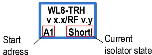
If the wired ESP loop has devices connected (for example, addresses 1 to 19 are occupied), you must change the start address (available from 1 to 127) to connect the following (wireless) devices:
