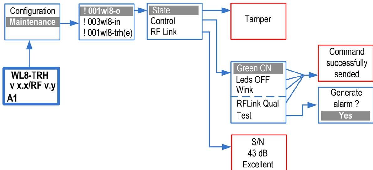
"!" at the beginning of the line means that there is a problem with a wireless device. By using the "State" menu, a user can obtain information about the general state (alarm/no alarm) and all current fault conditions of the device. Use the "UP" and "DOWN" buttons to scroll through the faults list.
