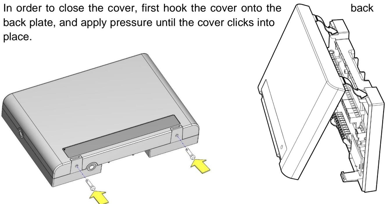
To secure the cover, you should insert the two rivet snaps into the holes.
