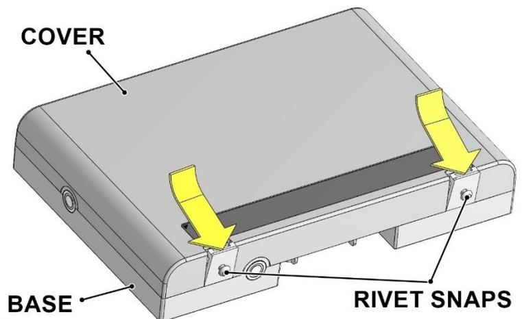
In order to close the cover, first hook the cover onto the back plate, and apply pressure until the cover clicks into place.
