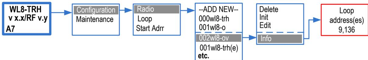
Devices that combine fire sensors and sounders (for example, EK-WL8-OS, EK-WL8-HS, EK-WL8-OV etc.) occupy two addresses on the ESP loop. The sounder within these devices will be addressed automatically by adding 127 to the sensor address and then using this number as the sounder address e.g. 9 (sensor address)+127=136 (sounder address).
