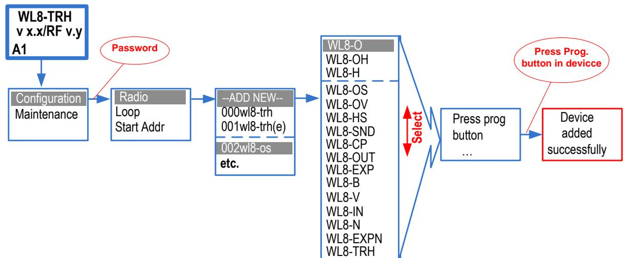
After the ADD command is performed, the translator waits for a device to be linked, to link a device press the device's "program button" (see the specific installation manuals of these devices).
