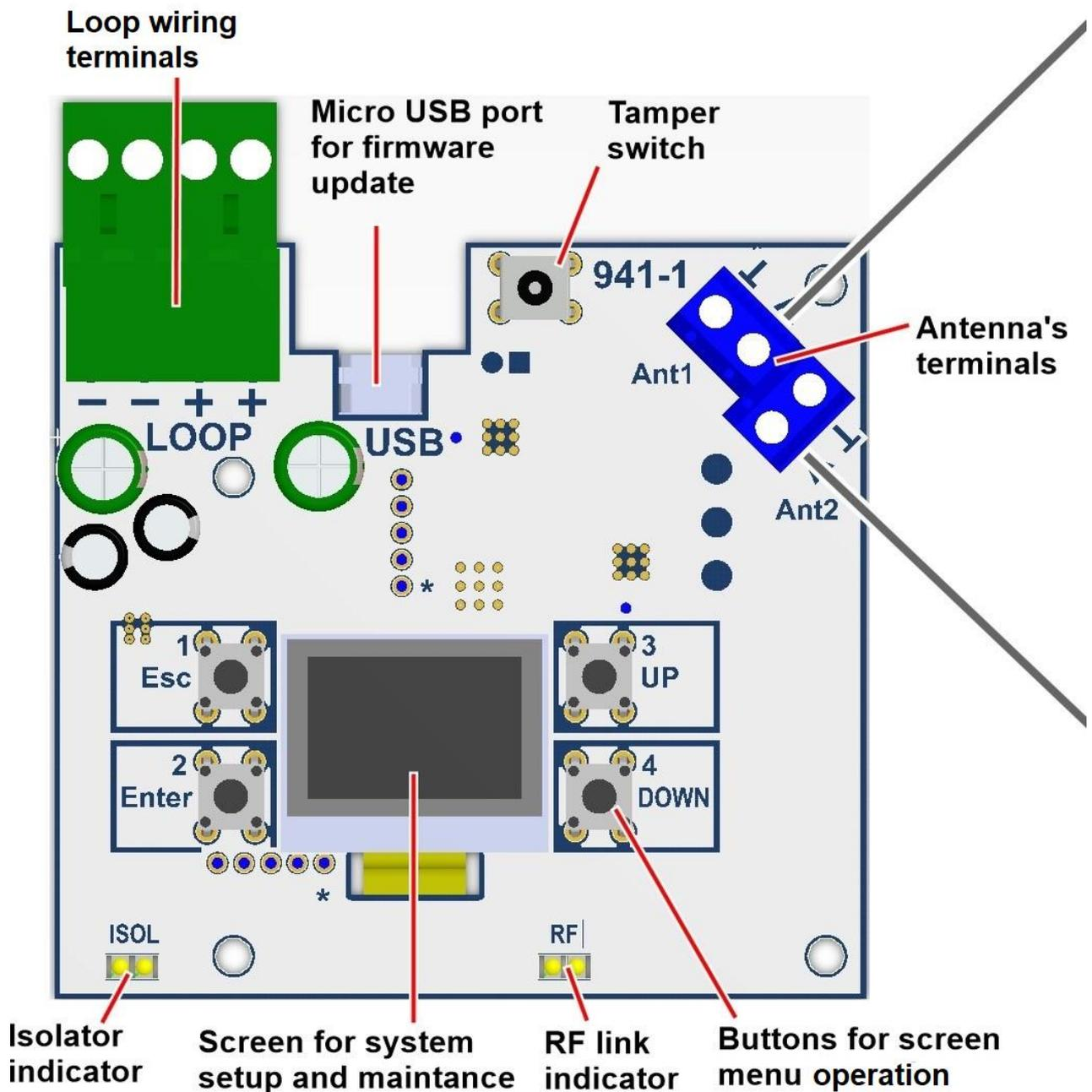
**LOOP WIRING TERMINAL BLOCKS:** Used for connecting the translator to the analogue loop
