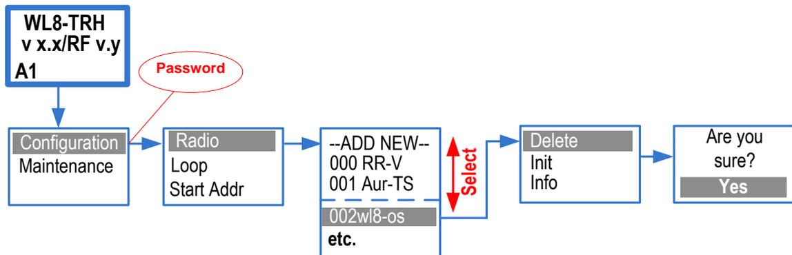
Be aware that this command deletes a device from the configuration of the translator, but not from the configuration of the main control panel.
